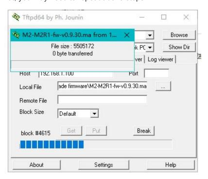
Step 11: The firmware has been uploaded but need to wait about 4 minutes for the router to finish storing firmware into its flash memory. Once it's done, you will see the Power LED will turn red and the wireless LEDs are both lit.
