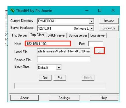
Step 9: Click the "Put" button on the tftp to perform a firmware upgrade.
