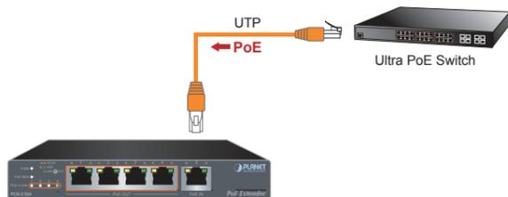
**Step 2:** The PSE delivers both Ethernet data and PoE power over UTP cable to the Gigabit PoE Extender.
