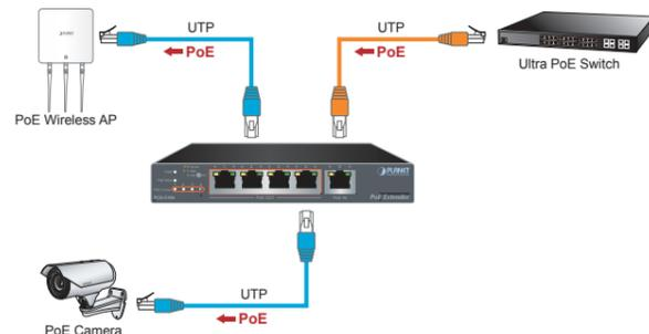
**Step 2:** The "PoE Out" port is also the power injector which transmits DC voltage to the Cat5e/6 cable and transfer data and power simultaneously between the PSE and PD.
