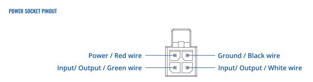
\*1/O: programmable Input/Output pins (Open Collector output max 30 V, 300 mA or Digital input where 0-6 V detected as logic low and 8-30 V - logic high).
