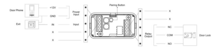
• Select Security Relay B for the SR01 to be powered by the third-party power supply. The relay is connected to the door phone via RS485.
