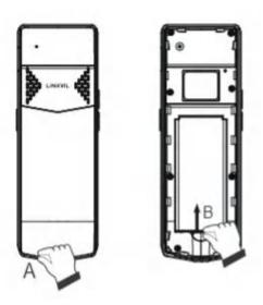
Remove the rear case Remove the battery
