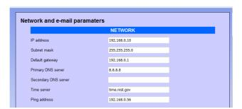
The default IP address of the device is **192.168.0.10**. Gateway and DNS are only needed if you want the device to have the ability to access the Internet (for example to get the current date / time, in the example from the site time.nist.gov).
