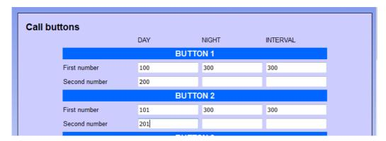
For each key, it is possible to enter for each mode of operation (day, night, interval), up to 2 contact numbers. If the software is unable to contact any of the numbers programmed, it is possible to transfer the call to another number, programmed in the "Supervisor":
