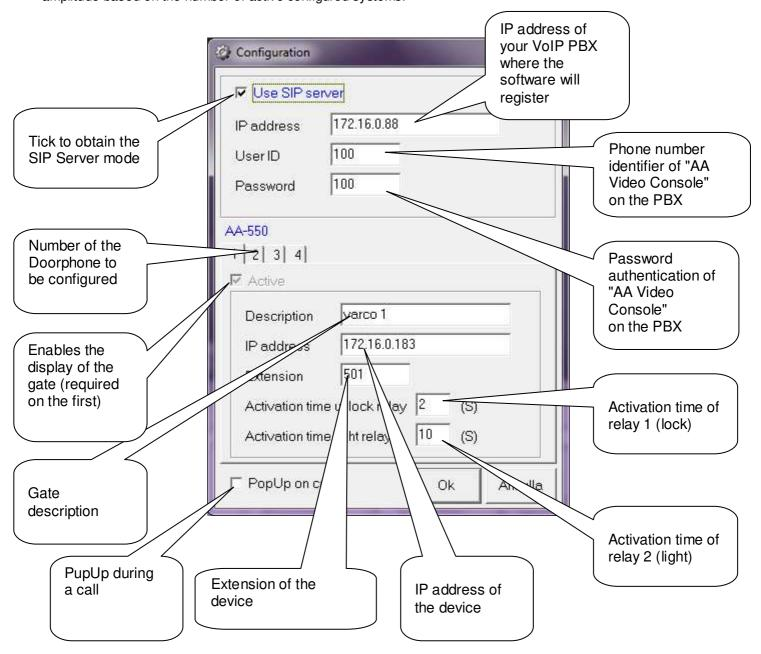
By customizing each description line for the operators will easily and immediately identify the system on the PC screen to be activated to perform the voice announcement from the PC microphone.
