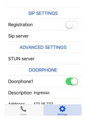
The first part, "SIP SETTINGS", allows to register your device to a PBX or a SIP provider (necessary if you want to reach the Doorphone through its extension number). Marking "Registration" you will have access to the account setup registration (user name, password, etc.). If into the network a SIP PBX is not installed and want to reach the Doorphone simply by its IP address, leave the check unmarked.
