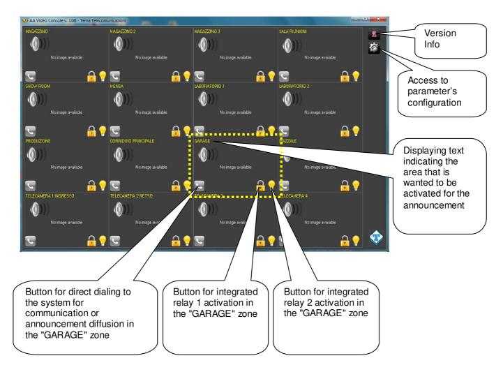
Pressing the handset icon, the program establishes connection with the related terminal and the operator will be able to spread his message by speaking into the microphone connected to the PC.
