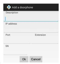
The extension number is the number that must be dialed when from the main screen is selected the call key. Obviously it makes sense only in SIP registered to the PBX Server. In Peer-to-Peer mode this field cannot be filled.
