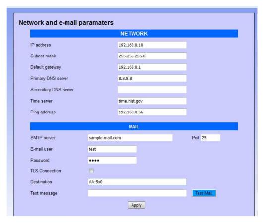
The default IP address of the device is **192.168.0.10**. Gateway and DNS are only needed if you want the device to have the ability to access the Internet (for example to get the current date / time, in the example from the site time.nist.gov).
