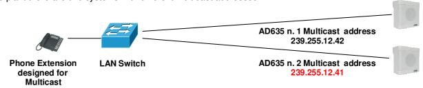
The phone, selecting to send the multicast voice to one or other address of the terminal, will decide which device must play the streaming message.
