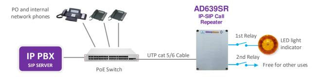
• SIP telephone call repeater with PoE injector or external 230Vac power supply
