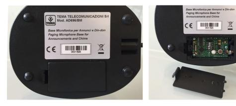
The board features programming dip-switches and two volume adjustment trimmers: one for adjusting the volume of messages announced via the microphone and the other for adjusting the start warning tones message (Chime). At the end of the adjustments or settings, replace the door in its seat.
