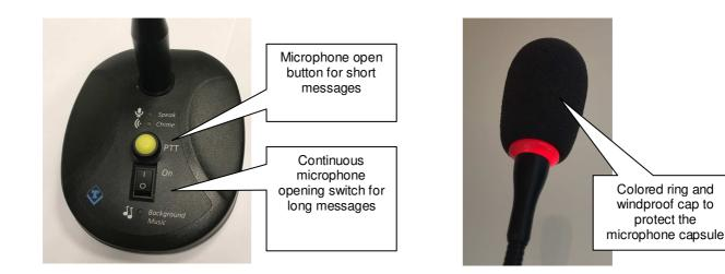
The operator who has the AD696/AA microphone base at his disposal, to issue an announcement on the speaker network after activating the "Microphone" function on the ADAM software window can:
