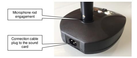
The other end of the cable will be connected to the audio system used, typically a sound card inserted into a computer where the ADAM software is running.
